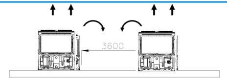
For mutliple chiller installation it is recommended to install the chillers is a single row as hown in the picture below
