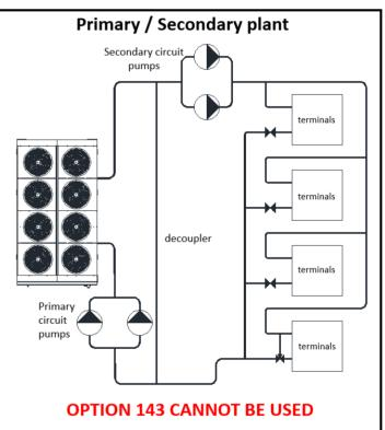
A bypass line (field supply) needs to be installed which guarantees that at all times the minimum water flow of the chiller is supplied (refer to the "Operating limit" chapter for indication on minimum water flow). The bypass valve will be an ON/OFF normally closed valve controlled by the chiller. In case the minimum water flow allowed is not reached, the chiller will open the bypass line restoring the water flow above the minimum value.
