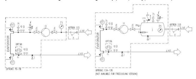
Hydraulic scheme of the Single V unit with Double Pump (max operating pressure 6 bar)
