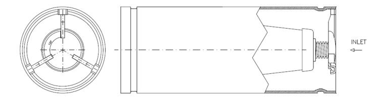
Water filter - Flanged connections (opt. code 153b) as alternative to Victaulic connection, same filters are available with flanged connections.
