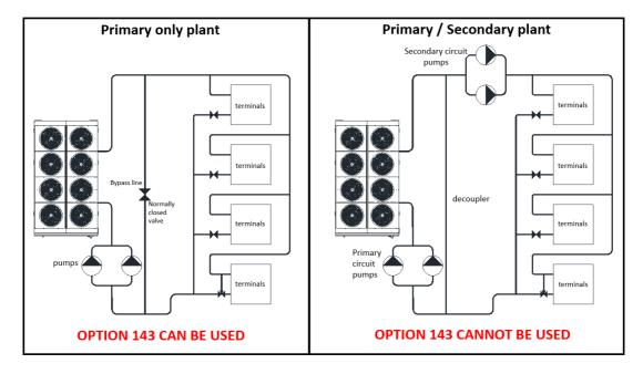
For unit installed in Primary/Secondary plants the option Variable Primary Flow is not applicable. In this case a different a different control is required.
