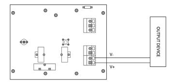
Wiring example for the relay switch output.
