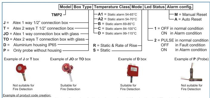
Heat detector ATEX certified T-box with glass, Temp. class C with alarm intervention at 90°C static with pulse LED and Auto Reset alarm:
