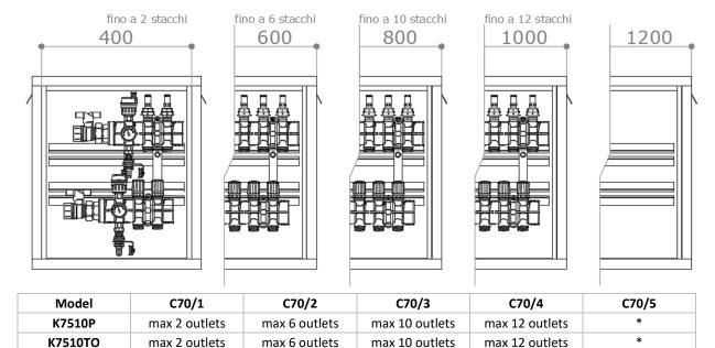
For the evaluation of the wall box size, the dimensions of isolating ballvalves and terminal group with drainer and automatic air vent have been taken into consideration; moreover, some free space has been kept for manifold installation and maintenance
