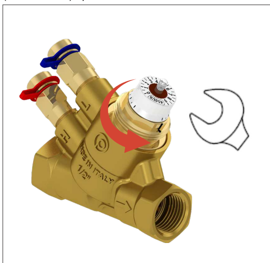
Step 2: using a 21mm (DN15 to DN25) or 30mm (DN32-DN40) spanner unscrew the headwork.
