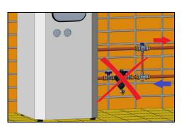
Upside-down and horizontal installation of the magnetic dirt separator MUST BE AVOIDED
