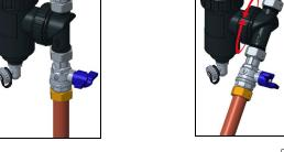
Thanks to the 360 ° swivel connection, using the specific provided key, installation on pipes that run vertically, horizontally or tilted is possible and easy. Avoid any installation position with the dirt separator axis is placed horizontally, diagonally or even upside down.
