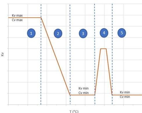
Working area 1 – Maximum Kv<sub>max</sub>, T<sub>water</sub> << T<sub>presetting</sub>
