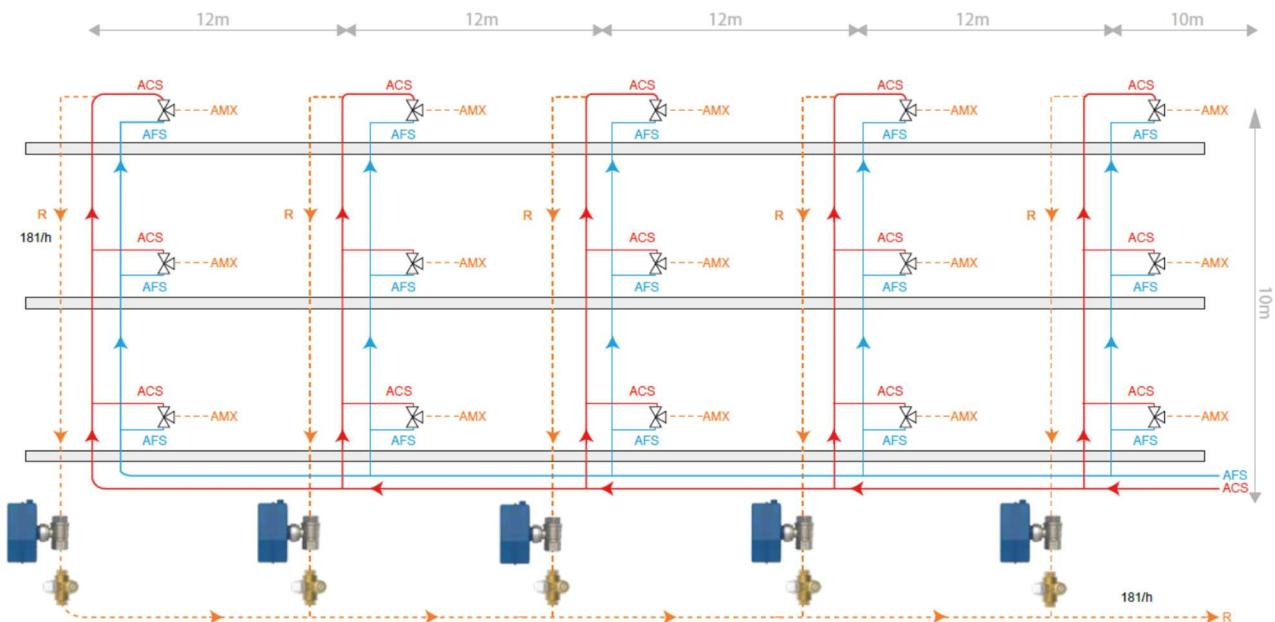
Once we have the flow rate for the least circuit (riser n° 5 – 181 l/h), based on the hypothesis of water temperature (75 °C) and maximum delta T allowed (5K) it is possible to proceed with evaluation of Kv and pressure drop at 70°C
