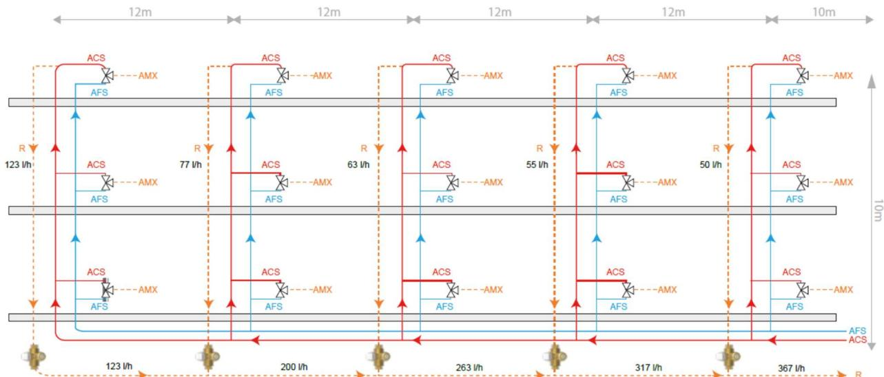
Once we have the flow rate for the least circuit (riser n° 5 – 123 l/h), based on the hypothesis of water temperature (75 °C) and maximum delta T allowed (5K) it is possible to proceed with evaluation of Kv and pressure drop at 70°C
