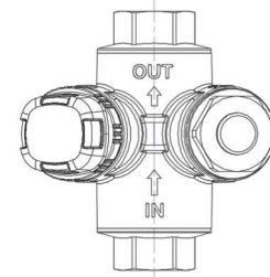
The TB30-TB30/2 thermostatic balancing valve can be installed without any particular precautions regarding the position; it can be installed both vertically and horizontally and possibly also upside-down. Not being equipped with built-in filters or electrical/electronic elements, there is no risk.
