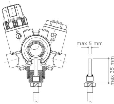
TB30 and TB30/2 has a drywell (1/2") that could be used (through an optional reduction OTB02 1/2" M x (M10x1)), to install a probe for remote monitoring of the water temperature.
