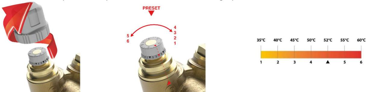
This is a simple but important operation for the proper functioning of the system. It is always advisable to preset the system valves at a temperature value greater than 3-5 ° C compared to the temperature actually desired on the most penalized users. This way, the overall pressure losses will be limited to the advantage of choosing the circulator dedicated to the recirculation network.
