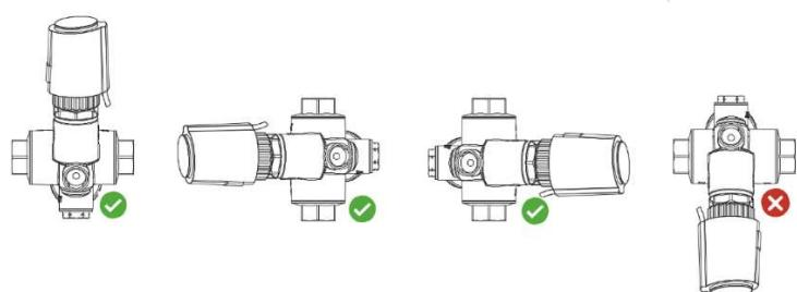
As for being the TB50-TB50/2 a valve that can be equipped with an actuator there is a need to follow some standard rules for the orientation of the valve:
