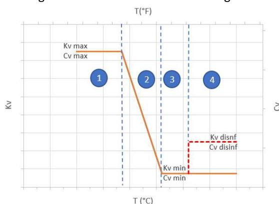
**Working area 1 – Maximum K<sub>vmax</sub>, T<sub>water</sub> << T<sub>presetting</sub>**
