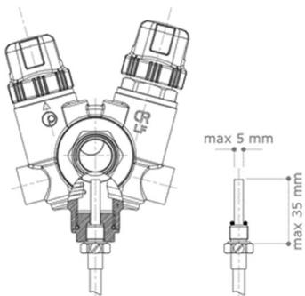
TB50 and TB50/2 has a drywell (1/2") that could be used (through an optional reduction OTB02 1/2" M x (M10x1)), to install a probe for remote monitoring of the water temperature.
