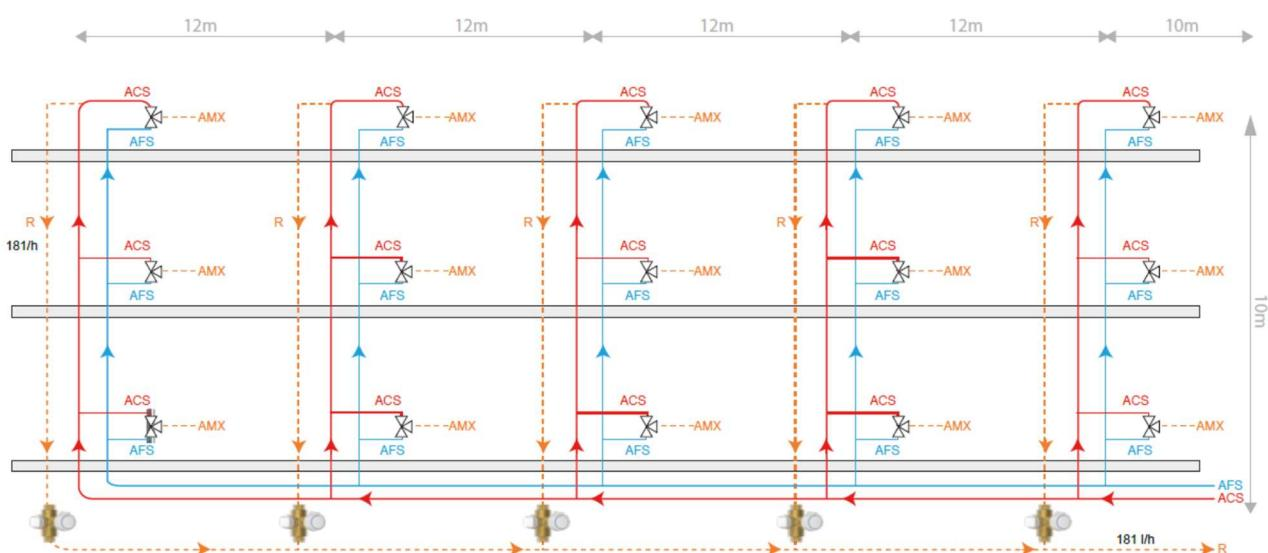
Once we have the flow rate for the least circuit (riser n° 5 – 181 l/h), based on the hypothesis of water temperature (75 °C) and maximum delta T allowed (5K) it is possible to proceed with evaluation of  $K_v$  and pressure drop at 70°C
