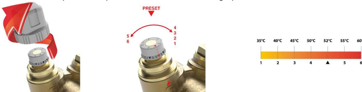
This is a simple but important operation for the proper functioning of the system. It is always advisable to preset the system valves at a temperature value greater than 3-5 ° C compared to the temperature actually desired on the most penalized users. This way, the overall pressure losses will be limited to the advantage of choosing the circulator dedicated to the recirculation network.
