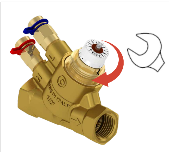
Step 8: Screw the headwork with 20 Nm torque
