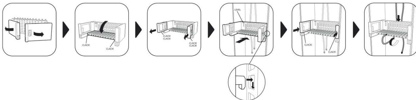
► Paso 2 : Instalar FLOW PSU
